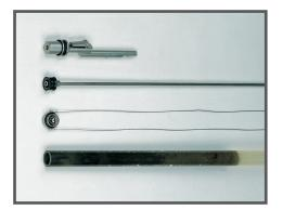
**Multisamplers** are used to take undisturbed samples of sediment and sludges.
