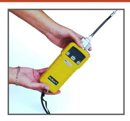
The **MiniRae 2000 PID** is a compact Photo Ionization Detector (PID).
