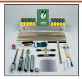
**Liner Sampler Sets** for collecting undisturbed samples for soil fertility, structure, volume weight, granular composition and technical determination in either soft or hard soils to a depth of 7m.
