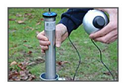
**e-Sense Telemetry Modem** a telemetric system with integrated datalogger with barometric & temperature sensors that fit inside 2-inch wells for a hidden and secure direct, remote monitoring solution.
