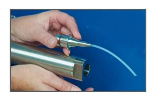
Bailers are a cheap and easy way to purge and or sample wells and open water.
