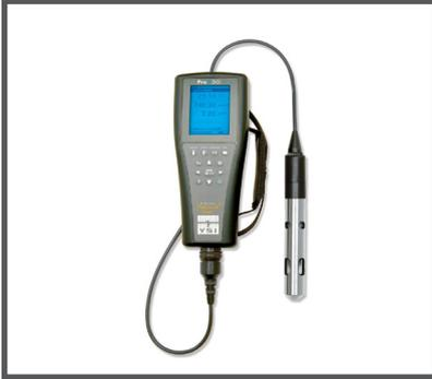
**YSI Pro ODO** is an extremely durable handheld Optical Dissolved Oxygen Meter.
