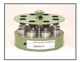
Wet Sieving Apparatus is used to determine the resistance of soil structure against mechanical or physicochemical destructive forces.
