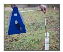
**Water Level Meter** is a reliable and accurate measurement of groundwater levels in boreholes, monitoring wells and tanks.
