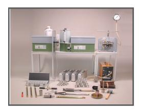
Sandbox set for pf determination when researching the quantity of water available in the soil for plants and trees.
