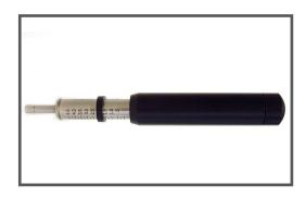
**Pocket Penetrometer** for the determination of the penetration resistance of an undisturded sample
