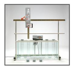
**Pipette apparatus** a simple method of determining the fractions of particles smaller than 38 microns in soil.
