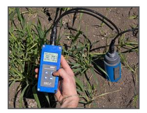
**Pico HD2 Meter** a mobile soil moisture readout device for accurate, clear onsite readings especially recommended for Pico 32 or 64 probes and tube profiling probe Pico IPH.
