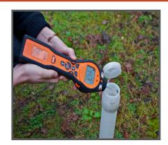
**Phocheck Tiger PID** a robust hand held VOC monitor with revolutionary PID technology that provides excellent detection and software features.
