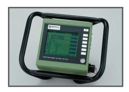
**Penetrologger** easy to use, lightweight electronic penetrometer for storage and processing of 1000 measurements.
