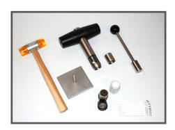
The **No Loss on-site Soil Corer** is ideal for taking exact 16ml samples of soil for testing volatiles using both the Methanol and Cooling methods.
