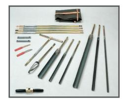
**Gouge Augers** are often used in cohesive soils to take undisturbed soil profiles down to 10 metres.
