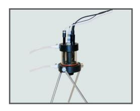
**Flow-through cell** to help and improve the accuracy of in-line measurement of pH, redox, EC, T, and  $O_2$ .
