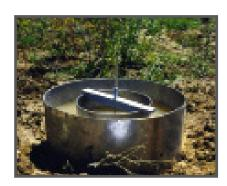
A **Double Ring Infiltrometer** is for the determination of the rate of infiltration of water into soil.
