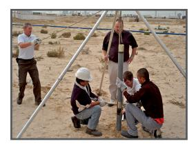
**Bailer Boring Hand Auger Set** for drilling above and below the water table to a depth of 7 meters.
